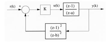
As can be seen in the figure, this loop has a reference input r(k), a control signal u(k), and an output signal y(k). The loop transmission has a variable gain K, three zeros at z = 1, one pole at z = a, and two poles at z = b. The zeros at z = 1 force the loop gain to be zero at DC.
